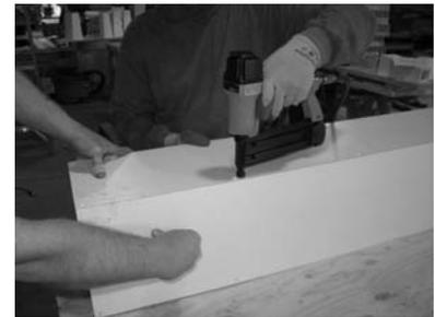
9) Or if you are not using screws, finish nail three panels together.
