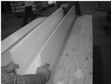
7) Assemble three panels, using E-Z lock joints.
