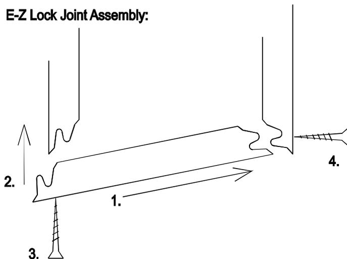
Please note the correct assembly of the E-Z Lock joint shown at the left. The screws or nails **MUST** be installed only in the edges shown (3 and 4). Installing on the other edges may result in open seams. (Pre-drill if using screws.)
