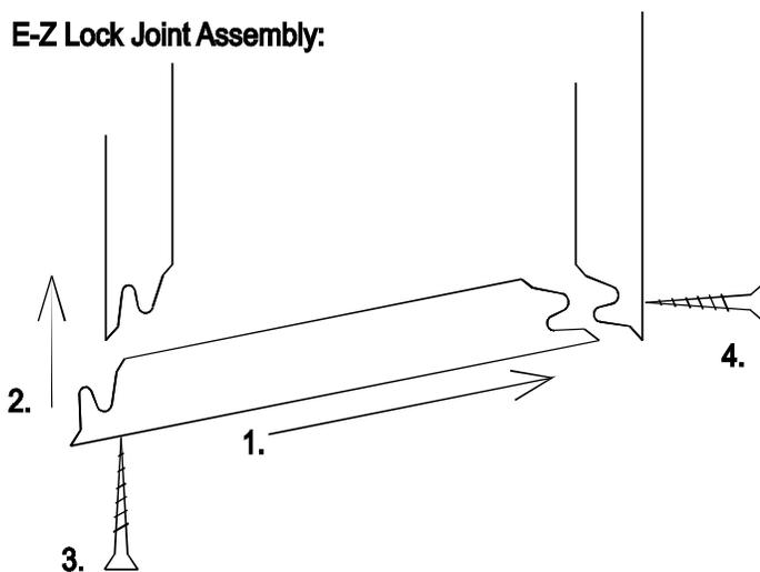
Please note the correct assembly of the E-Z Lock joint shown at the left. The screws or nails **MUST** be installed only in the edges shown (3 and 4). Installing on the other edges will result in open seams. (Pre-drill if using screws.)
