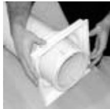
12. Slide cap over the top of the column to rest on the neck ring, then slide the base onto the column.
