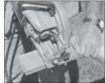
4. Trim wood inserts 1/4" shorter than PVC rails. (PermaRail fastening kits are 1/8" thick. One for each end). Trim aluminum inserts to opening measurement.
