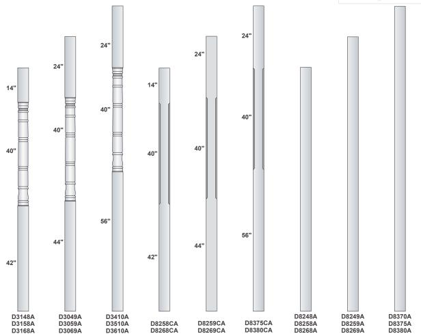
Net width is 3/4" less than nominal. Inside width of 5" posts is 1 3/4", inside width of 6" post is 2 3/8". All styles are available in 8', 9' and 10' heights. See chart below for available widths. Posts are load-bearing (unless split.)
