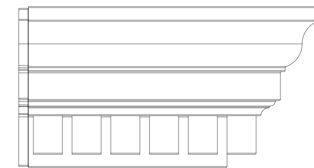
ELEVATION OF CR-115X8 OUT CORNER SCALE 1:1
