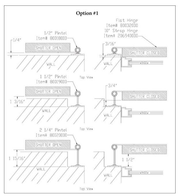
The ideal setup is to have the Shutter flush with the casement when the Shutter is in the closed position. The Pintel Shims can be added to make small adjustments of 1/4", 1/2" and 3/4".
