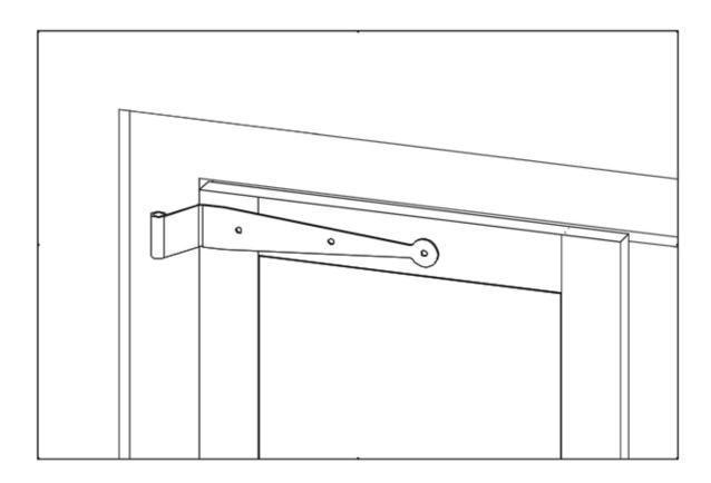
With the Shutters setting in the window opening, attach the Strap Hinge to each Pintel and rotate the Hinge to lay flush with the face of the shutter. Mark the location of the screw holes.
