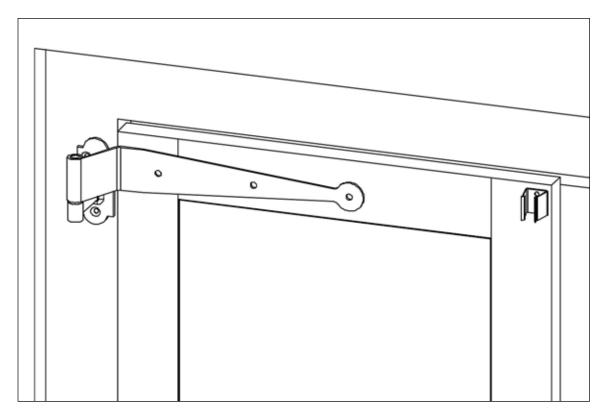
Swing the shutter open and mark the location for the Acorn Clip on the wall. If mounting in a wood surface drill a 1/4" pilot hole and mount the Acorn Clip. If mounting in a masonry surface use the appropriate anchor.
