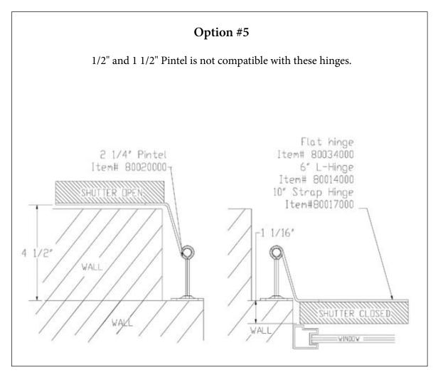
The ideal setup is to have the Shutter flush with the casement when the Shutter is in the closed position. The Pintel Shims can be added to make small adjustments of 1/4", 1/2" and 3/4".
